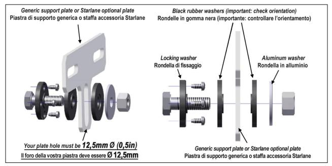
In particular the hole in the bracket must be drilled in **12,5mm (0,5in)** diameter, **and not 8mm**, in order to allow <u>the protruding side of the rubber washers to fit in the inner side of hole between the bolt</u> and the bracket,
